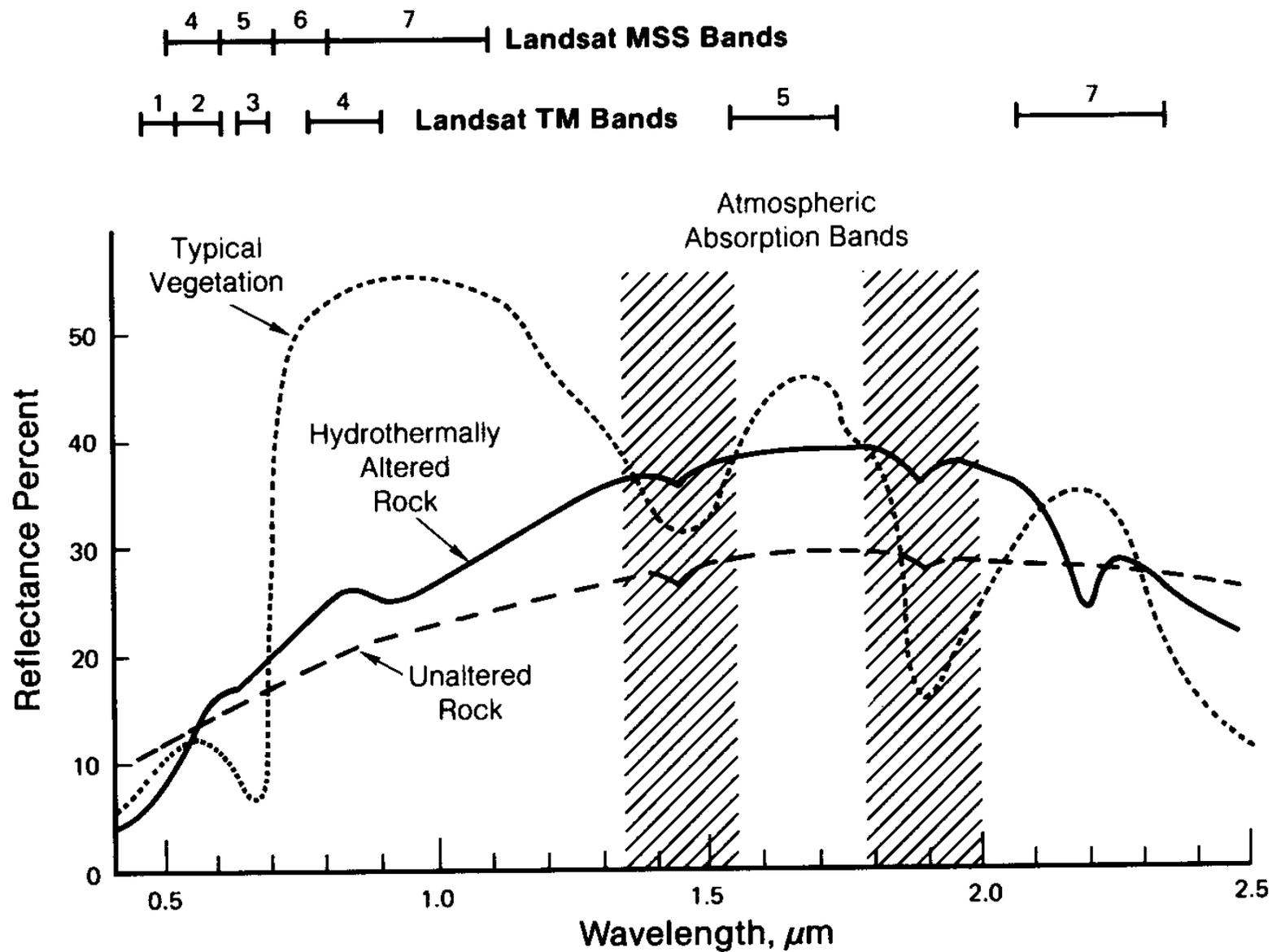
**FIGURE 4.14** Spectral bands for TM and MSS systems. Reflectance curves for vegetation, unaltered rocks, and hydrothermally altered rocks. From Sabins (1983, Figure C-5).
