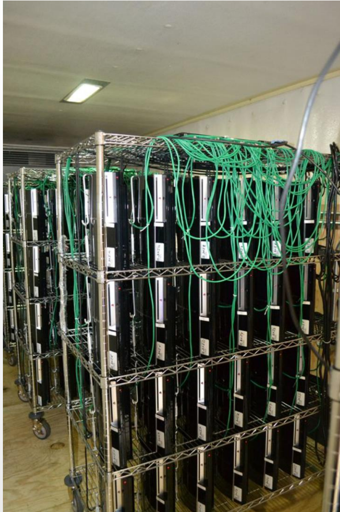
A PS3 supercomputer at UMass Dartmouth. Photo by Gaurav Khanna / UMass Dartmouth
